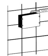
After you have chosen the ideal location for your sensor flush plate. Use the control panel base to mark where you wish to install the flush plate.
